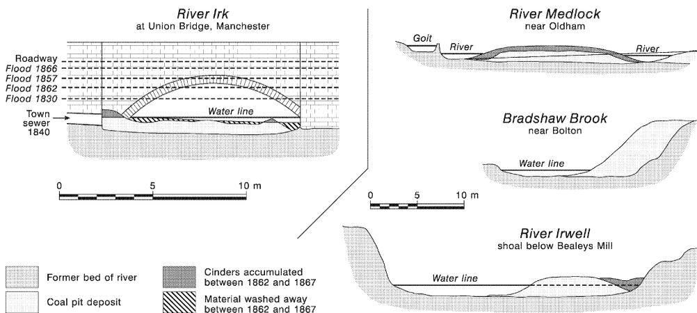
Fig. 7. Mid-19th century changes to river channels due to the dumping of cinders and other wastes, as described by the Royal Commission on Rivers, 1870. Note particularly how siltation of the Irk at Union Bridge had buried the outlet of the town sewer at least 1 m below a mass of debris. (Source: Rivers Pollution Commission, 1870).
